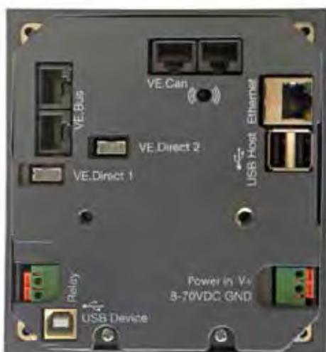
When more than two VE.Direct products must be connected, USB can be used.
