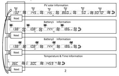
**Data setting instructions:** on reading display, press K4 for setting and next data, then save it. K1 for next data, without save. K2 and K3 for modify the data, shows as following picture 3.
