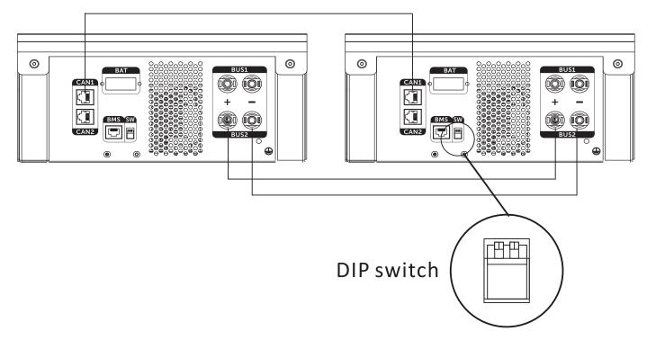
Please set DIP switch when install the expanded BMU. For SK-SU, the internal BMU is recognized as C1, and the expanded BMU is recognized as C2-C4.
