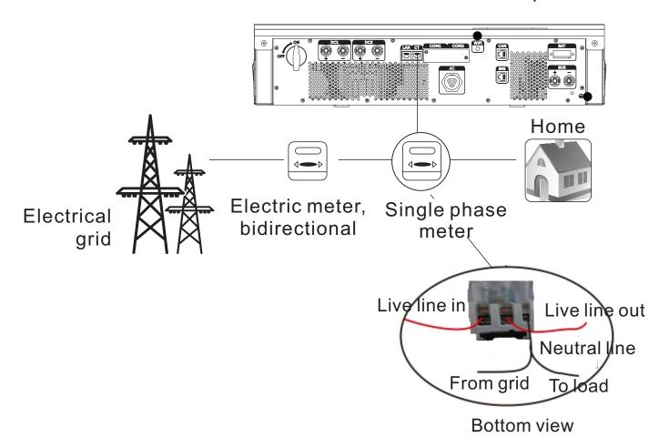
2. Connect power meter to the inverter with communication cable. It comes with meter.
