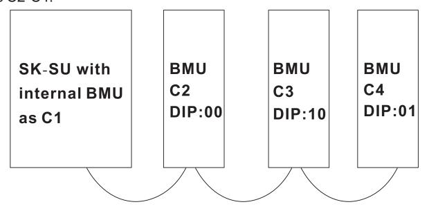
For DIP switch, on the up position refer to "0", and on the down position refers to "1".
